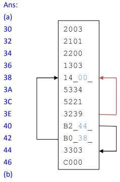
If 3239 is replaced with 3238, it will change the OP code which is in the "38" address of memory. Then the program logic will be wrong.
